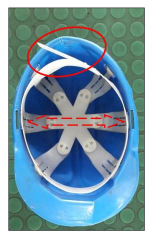
Figure 4: Deformed and damaged safety helmet
