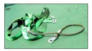
Figure 4: The fall arrester in use at the time of the accident
