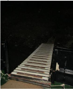
Gangway has not been manufactured by recognised international standards, is not properly secured, has no side screens or handrails provided and is not well lit.
